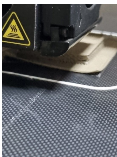
Figure 29 - Printing using SERTENE PPx200C RC
