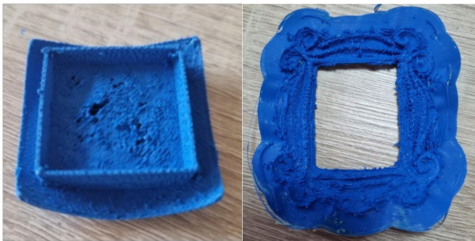
Figure 32 - Element made with light blue flakes from K-FLEX
