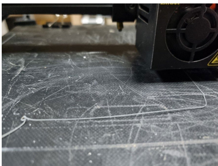
Figure 31 - Peeling off the object during the printing using SERTENE HDRPO 0100
