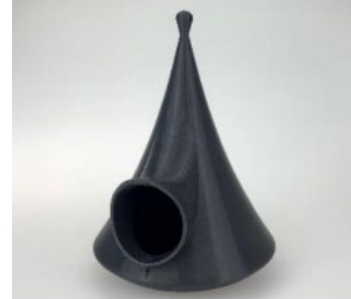
A figurine printed from recycled polylactic acid filament, or R PLA, by Fiberlogy (©Fiberlogy)
