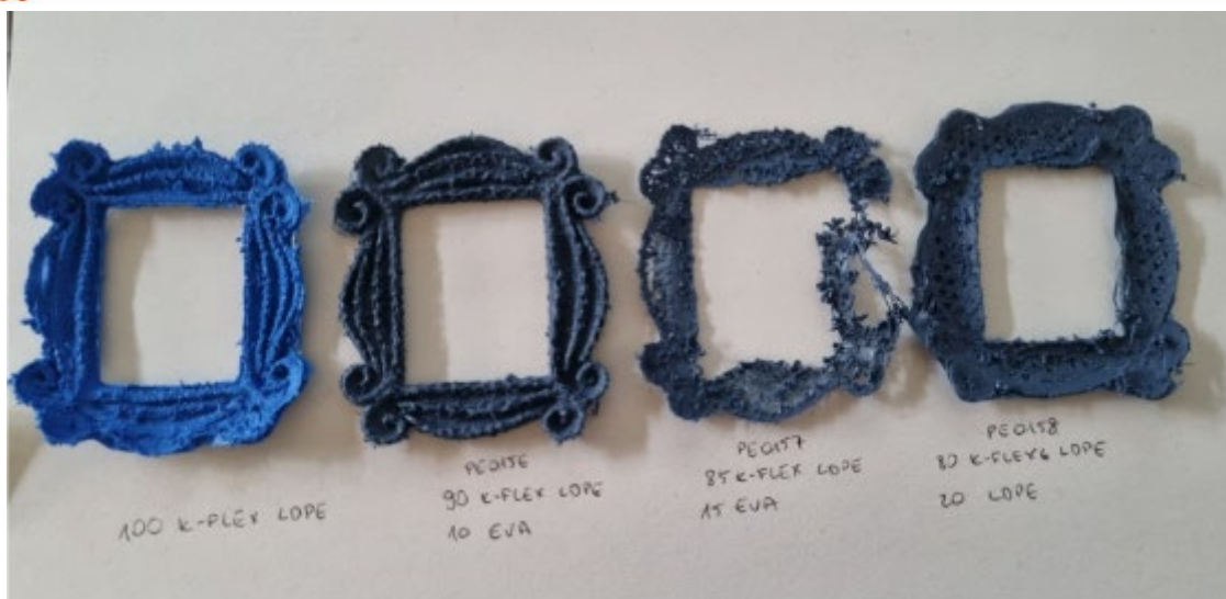
Figure 34 - Elements made with blue granulate from K-FLEX with pure polymers
