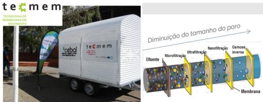
Figure 43: Mobile membranes unit developed within the TeCMEM project.
